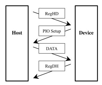
Figure 5.15 PIO data-out command protocol
